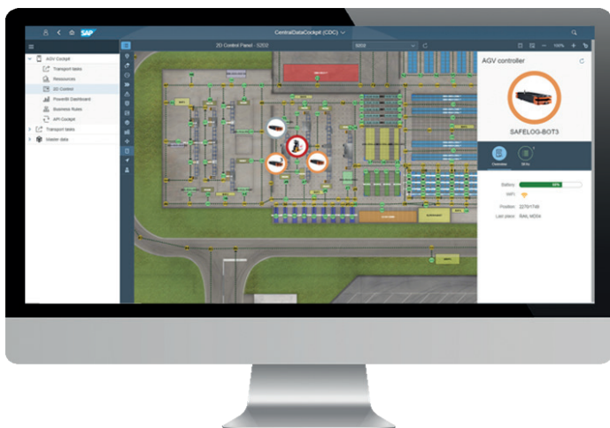
CDC (Central Data Cockpit): Overview and live locations of all AGVs in your company as well as current status and fault messages at a glance.
